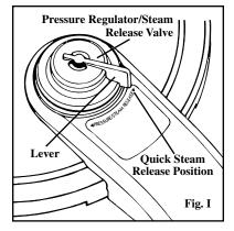
B) Cool the pressure cooker under a running water faucet or pour cold water over it until pressure is completely reduced. Pressure is completely reduced when the air vent/cover lock has dropped. Note: Do not set hot cooker in a molded sink as it could damage the sink.
